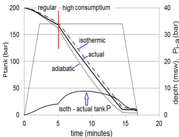
Fig. 1 Simulation to 34 msw. Regular AC is 17 aL/min and high is 43 aL/min. The 3 upper curves give the tank pressure for the 3 conditions. The lower one the adiabatic effect on tank pressure (the “extra” air).
