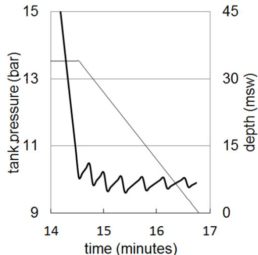
Fig. 2 Tank pressure during ascent from the 34 msw when the first stage blocking pressure (10 bar) is reached and the emergency ascent starts.
